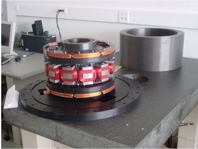
Figure 8. A magnetically suspended high speed flywheel being developed at LaunchPoint Technologies.
